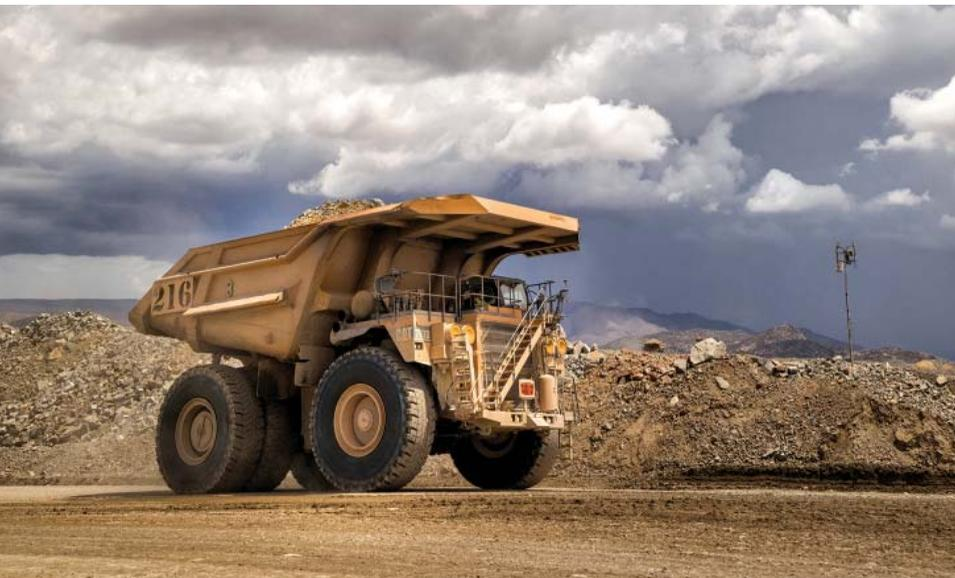
As each haul truck comes into the shop for a rebuild, it will be converted to AHS. (Photo: Freeport)
