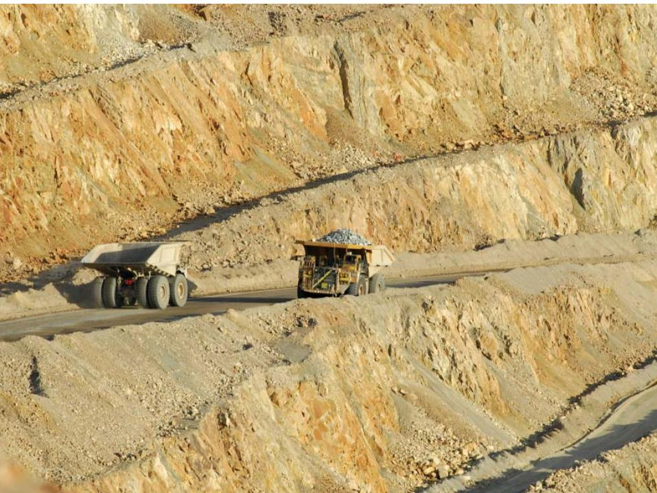
The cycle time for the trucks at Bagdad varies from 30 to 60 minutes from the pit bottom to the crusher or multiple waste dumps. (Photo: Freeport)
