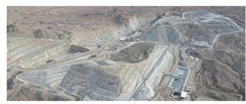
An aerial view of the Moss mine looking east shows the West and East Pits and the crushing installation in the center. (Photo: Elevation Gold)
