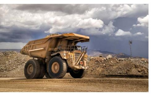
As each haul truck comes into the shop for a rebuild, it will be converted to AHS. (Photo: Freeport)
