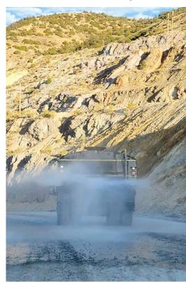
Pinto Valley uses a 1:1 ratio of magnesium chloride to water in its water trucks to suppress dust. (Photo: Capstone Copper)
