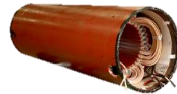
Pleuger: 500HP 4160V 1750 RPM 19 Inch Case Water Filled
